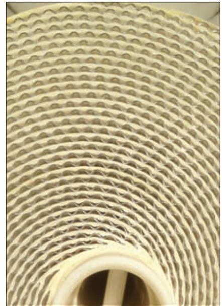
Figure 5: iSep UF flow channels
