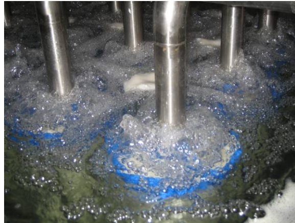
Figure 4. Membrane aeration process.
